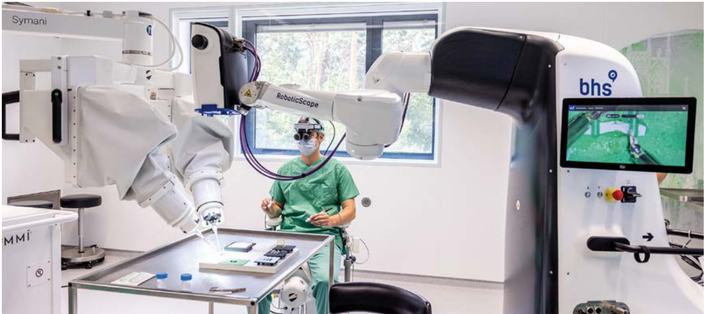
Prof Maximilian Kückelhaus presents the new method in a "dry run" in a training session. The surgical robot (left) is linked to a robotic microscope (right).
